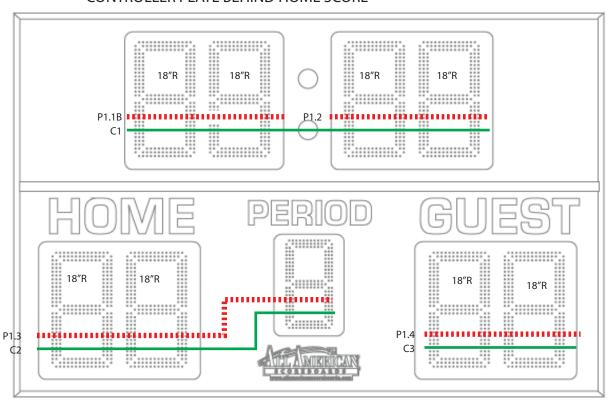
Power Supply Outputs (Full Brightness & Full Digits):  $P1.1 \approx 2.98A$   $P1.2 \approx 2.38A$   $P1.3 \approx 3.48A$   $P1.4 \approx 2.38A$  "C" refers to controller board output. If Indicators are used, C4 data will go to the Indicator Driver Board and then to the digit(s).
